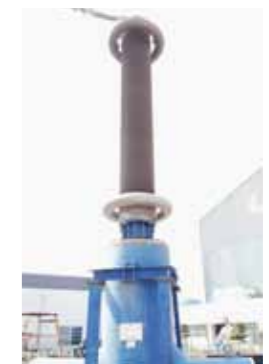
[L-series test termination]
